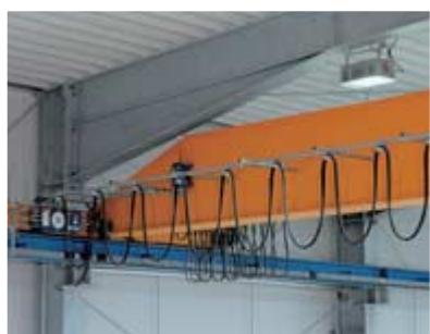
The ideal solution for a new factory: the ABUS ELK single girder travelling crane with long angle chamfer adapted to suit the building haunch (version 3), optimising available height.
