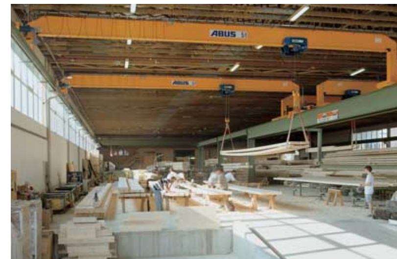
ABUS single girder travelling cranes can be equipped with different girder connection versions for each track. In this way, you can divide a wide factory into two sections, allowing highly flexible material handling.
